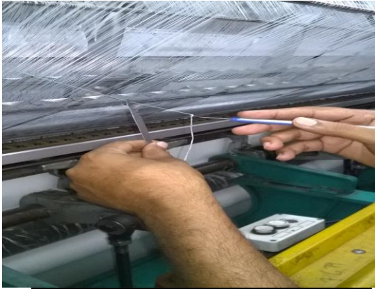
3 Broken thread gripped by hook
