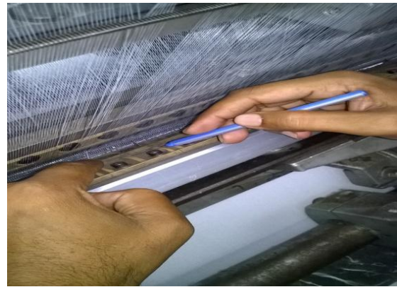
6 Thread passed through guides
