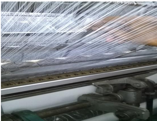
7 Thread passed through guides
