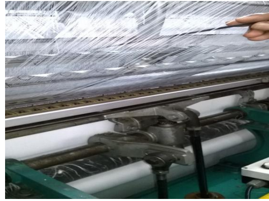
4 Thread passed through guides
