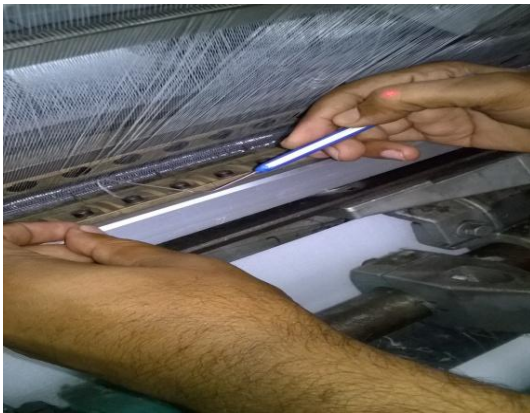
5 Thread passed through guides
