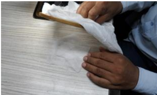
Putting the fusing material beneath the fastened fabric in the frame
