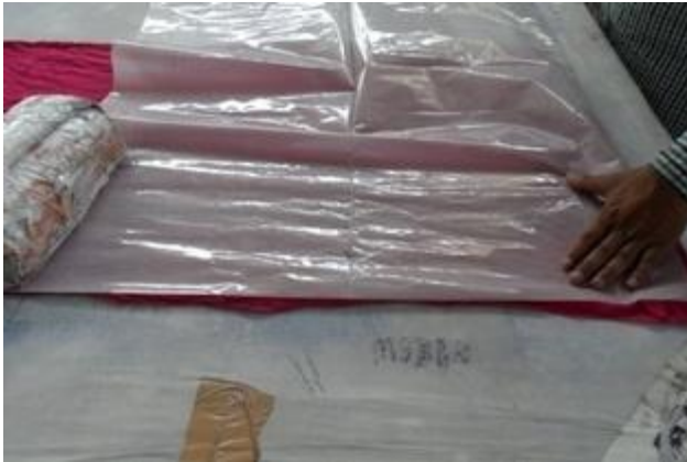
Putting the design pinned tracing paper on the fabric
