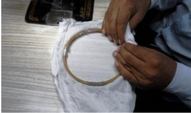
Putting the frame to fasten the selected fabric area
