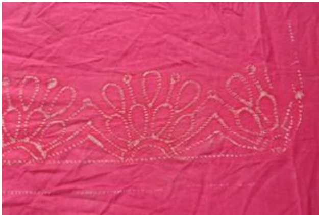
The design is transferred by using the powder pigment on to the fabric
