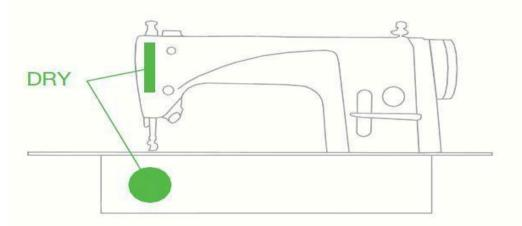
The section around the needle bar, the thread take-up lever and the hook are not lubricated.
