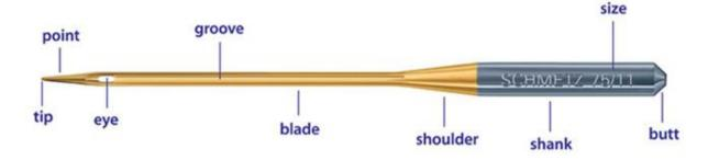
There are two needle sizing system :American and European. American Needle sizes range from 8 to 19, and European sizes range from 60 to 120. Larger the number, the larger the blade of the needle.
